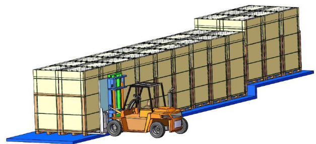
Long-side vertical package unloading with forklift
