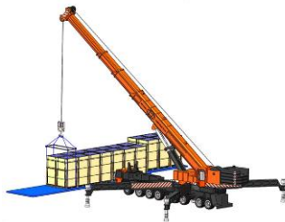
Long-side vertical package unloading with crane
