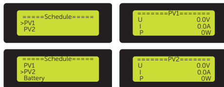
Figure 9-14 Displaying PV1 and PV2 status
