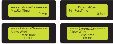
Figure 9-83 Setting MaxRunTime, MinRestTime, allow working period
